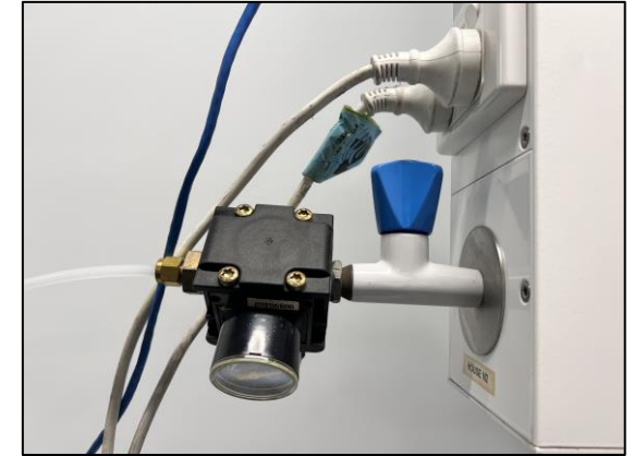
Nitrogen supply for CAD detector. Rotate the blue knob to open or close the gas supply.
